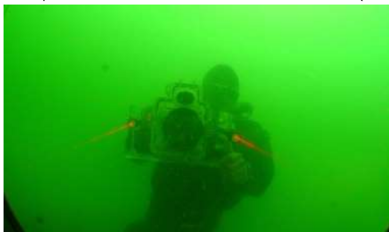
Fig.2. Underwater camera with the laser pointers
